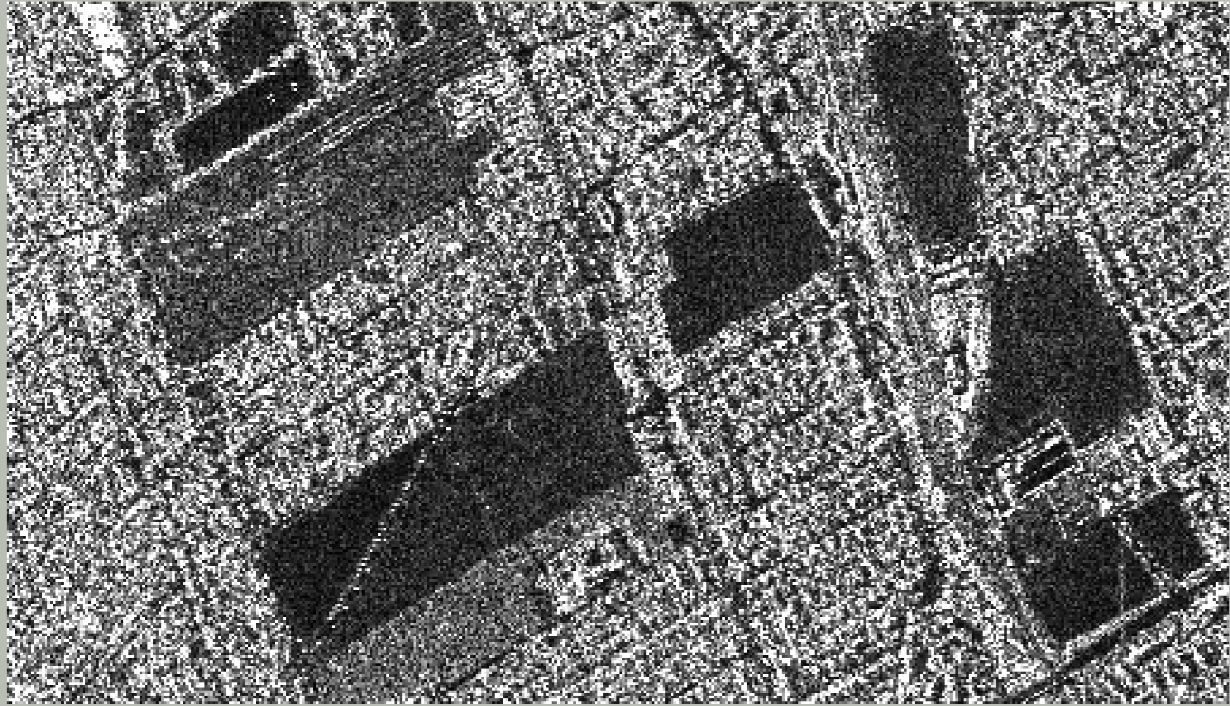
Figure: Speckle, non additive and non gaussian noise. The noise is multiplicative and \mathcal{G}^0 distributed. Real image, Munich city
